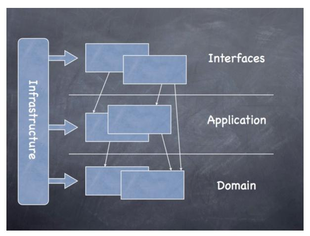
As you can see, there are three vertical layers: interfaces, application, and domain, each supported by different kinds of infrastructure. In the application, the package naming reflects these layers.
